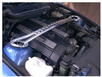
the studs will be flush with shock tower- loosely attach opposite side bar and nuts, then carefully lower car so other side studs will raise up through bar holes into proper location.
